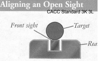
Sight correctly aligned on target
