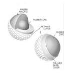
The modern golf ball consists of rubber thread wound around a rubber core and coated with dimpled enamel. The dimples are arranged in rows. The number of dimples is either 336 for an American ball or 330 for a British ball.
